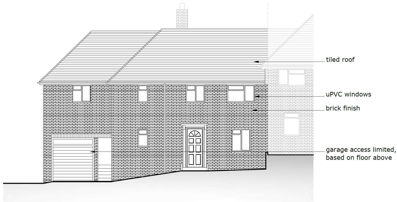
existing north east elevation 1:100
