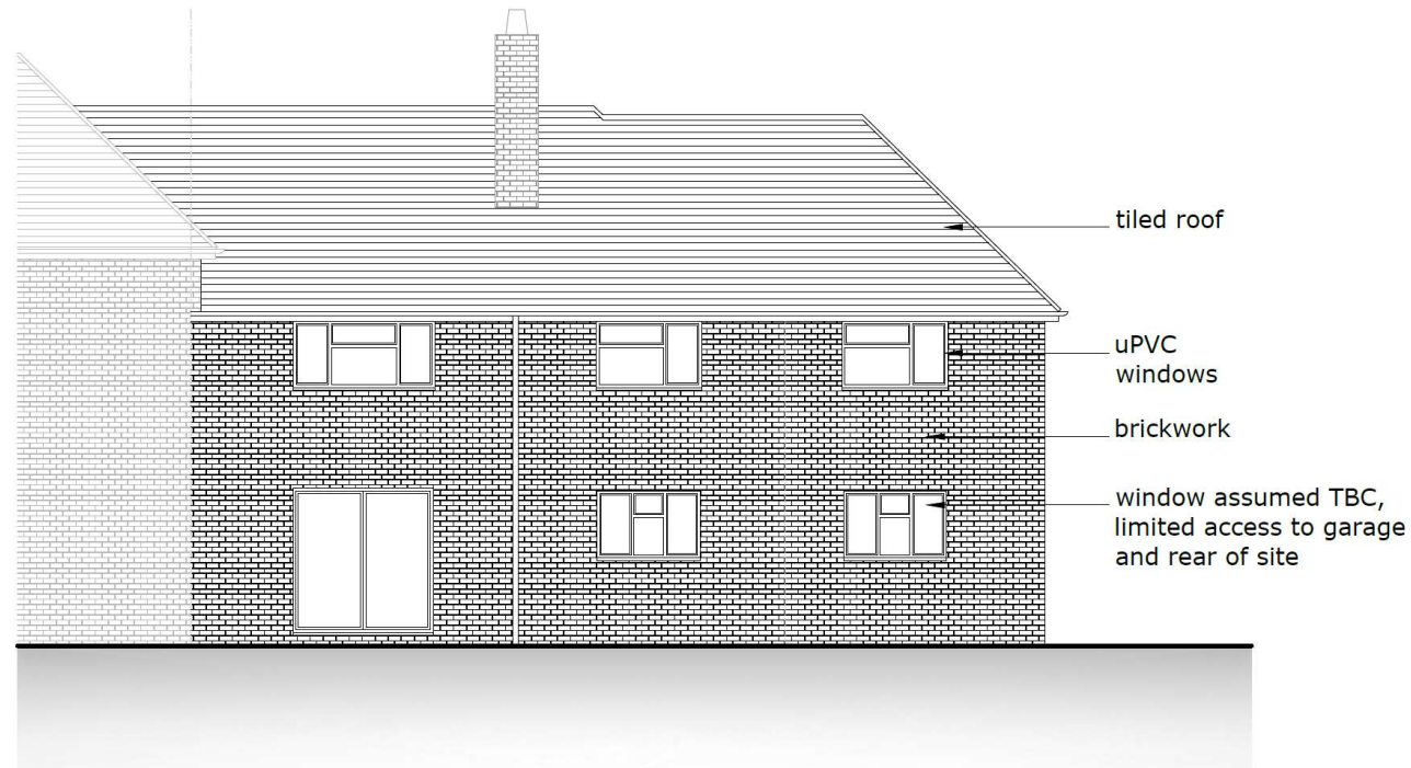
existing south west elevation 1:100
