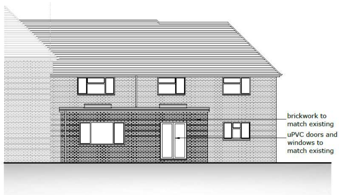
proposed south west elevation 1:100
